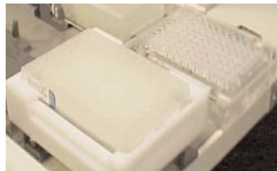
Figure 4. Vacuum manifold disassembly, placement of Elution Plate and reassembly of vacuum manifold for elution of purified amplification products on the Beckman Biomek® 2000.
