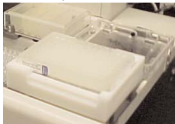
Figure 4. Vacuum manifold disassembly, placement of Elution Plate and reassembly of vacuum manifold for elution of purified amplification products on the Beckman Biomek® 2000.
